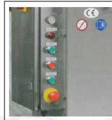
Pushbutton control for bowl elevators and tippers
